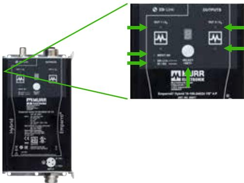
IP67 power supply **diagnostics** are visible directly on the device, taking advantage of a visible status LED. Whereas when using IP20 power supplies inside enclosures, diagnostics information is difficult to access. To get the same diagnostics information with an IP20 power supply, you would need to open the enclosure (results in higher costs, reduced IP protection).
